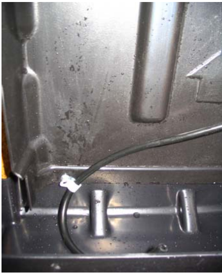
Insert the 36"(900mm) tube in the tube-attachment.
